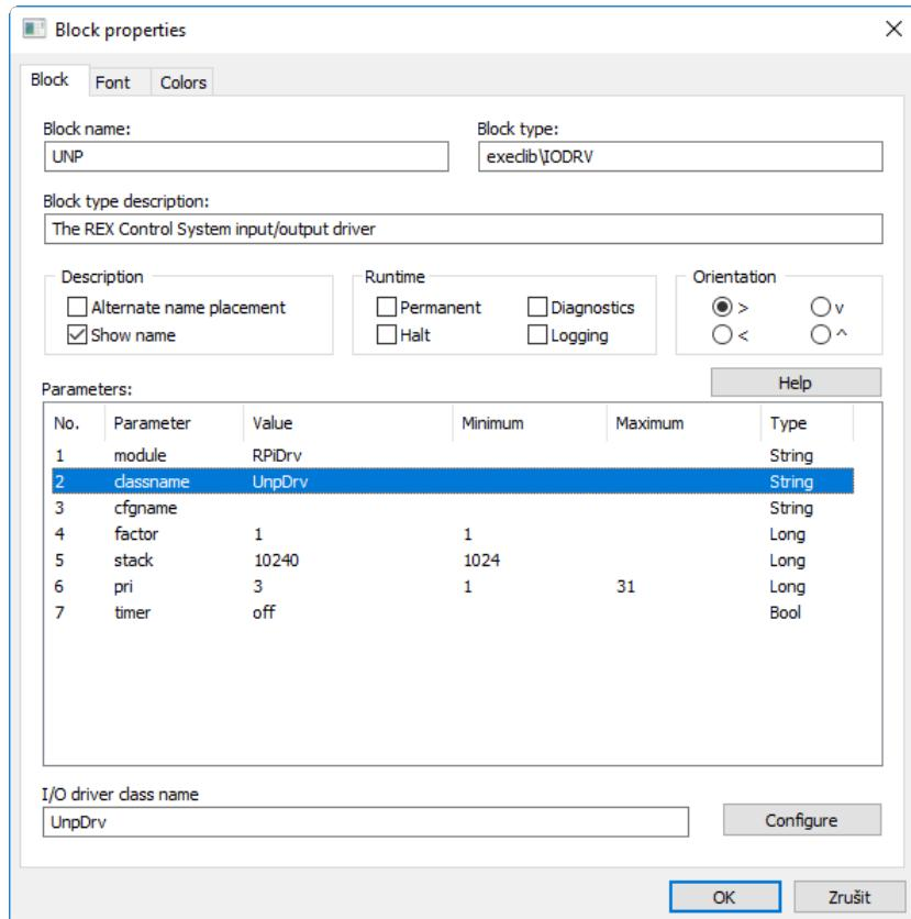
As the final step, rename the IODRV block to UNP, which will serve as a prefix for all I/O signals of this driver.
