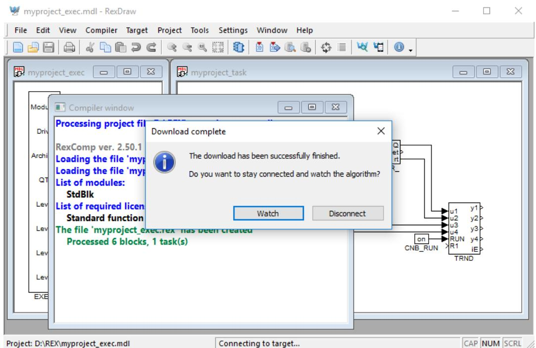
The RexDraw program now works in the so-called online mode. Right-click the TIMER\_BLOCK block and select **Monitor selection** in the menu to watch the inputs and outputs of the timer.
