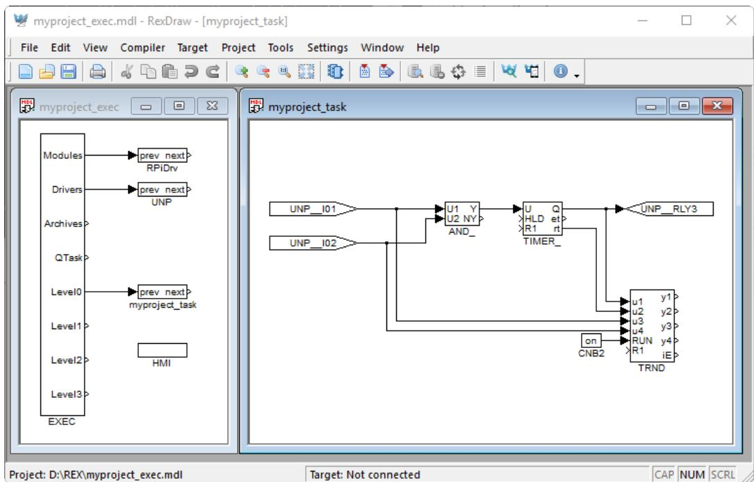
After compiling the project and downloading it to the Raspberry Pi the control algorithm interacts with the physical world. Again it is possible to switch to online mode and watch the signals in real-time or analyze the trends of signals. Flip the physical switches and watch the signals.
