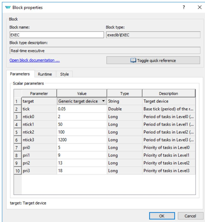
6. Note that `tick=0.05` and `ntick0=2`, therefore the task will run each 100 milliseconds ( $0.05 \cdot 2 = 0.1s$ ). There is no need to change any parameter at the moment. Close the dialog.
