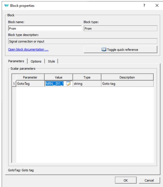
The other physical switch (SW3) is connected to Digital Input 1.3 (NRN\_\_DI1\_3). The last (Digital Output) flag will be set as `GotoTag = NRN__D01_1`
