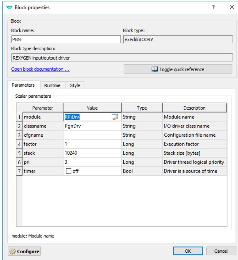
As the final step, rename the IODRV block to PGN, which will serve as a prefix for all I/O signals of this driver.
