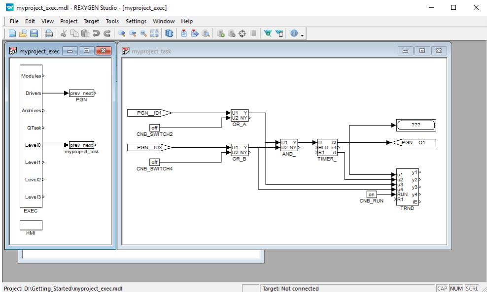
After compiling the project and downloading it to the Pigeon PLC the control algorithm interacts with the physical world. Again it is possible to switch to Watch mode and observe the signals in real-time or analyze the trends of signals. Flip the physical switches and watch the signals.
