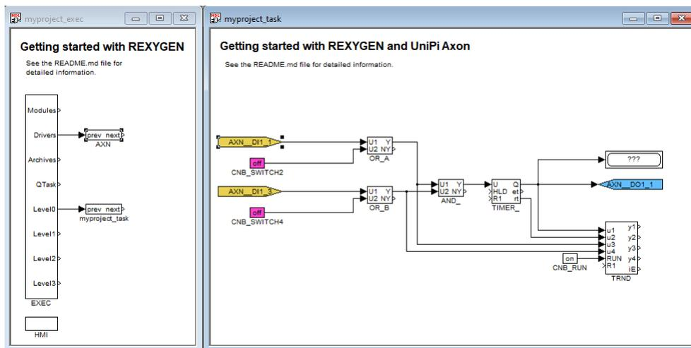
After compiling the project and downloading it to the UniPi Axon/Patron the control algorithm interacts with the physical world. Again it is possible to switch to Watch mode and observe the signals in real-time or analyze the trends of signals. Flip the physical switches and watch the signals.
