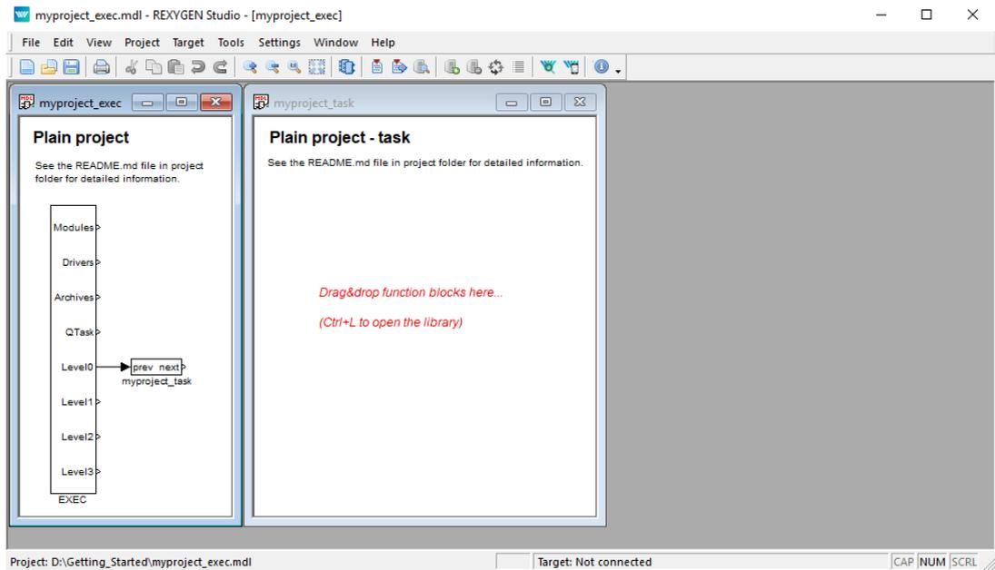
4. The task is connected to the `Level0` output of the `EXEC` block and therefore its timing is defined by `tick` and `ntick0` parameters of the `EXEC` block.
