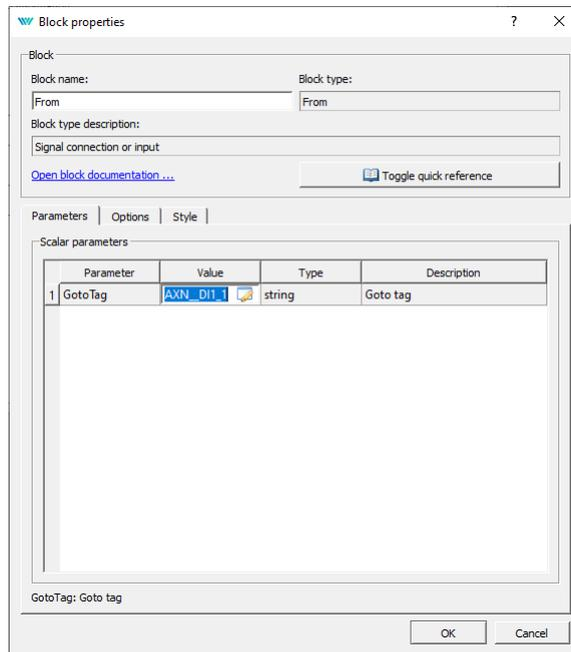
The other physical switch (SW3) is connected to Digital Input 1.3 (AXN\_DI1\_3). The last (Digital Output) flag will be set as `GotoTag = AXN_DO1_1`. Your project should now look like this:
