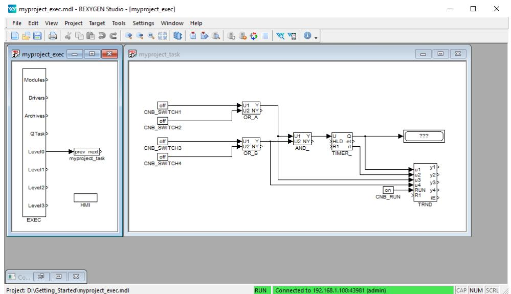
3. Double-click the HMI block to edit its parameters. Set `GenerateWebWatch = off` and confirm. WebWatch is another type of HMI, which you do not need at the moment. See [5] for details, it is a very interesting tool for developers and technicians.
