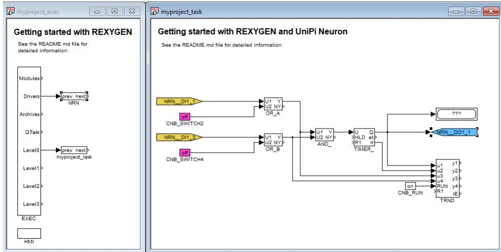
After compiling the project and downloading it to the UniPi Neuron the control algorithm interacts with the physical world. Again it is possible to switch to Watch mode and observe the signals in real-time or analyze the trends of signals. Flip the physical switches and watch the signals.
