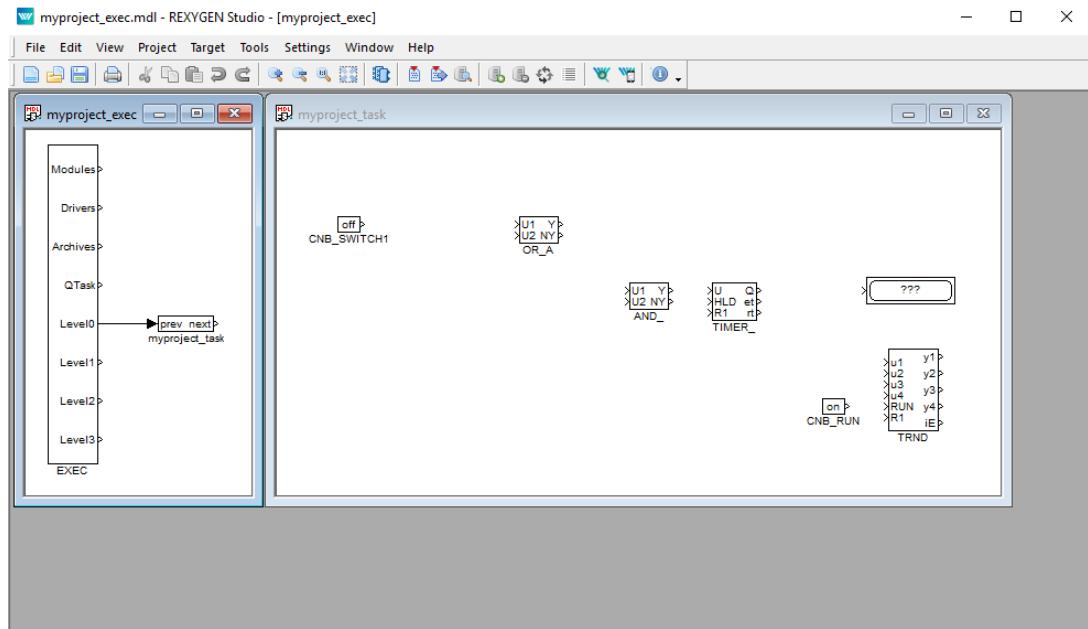
12. Duplicate the **CNB\_SWITCH1** block with right mouse button dragging. Or simply Copy&Paste the block.
