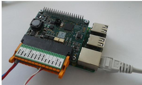
Figure 3.2: Terminal pinout for Monarco HAT.
