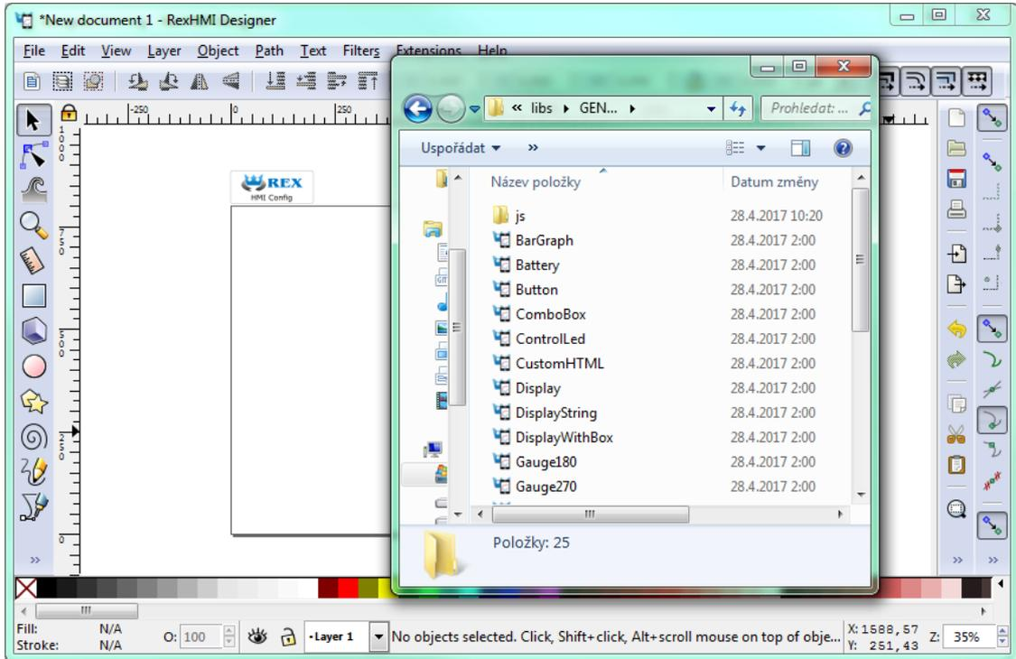
For configuration of the display settings select the display by mouse click on top of it and use the *Edit Component* extension from *Extensions* → *RexHMI* → *Edit Component* (Ctrl+E). When the configuration dialog is opened you can change the *Title* to *Display\_remaining*. The Edit Component dialog has two tabs: *Data points* and *Options*.
