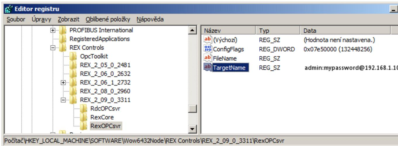
Afterwards it is possible to establish data exchange with the running executive of the REX Control System from the visualization software. The OPC server named REXControls.RexOPCsvr allows the visualization SW to read all inputs, outputs and parameters of the function blocks the control algorithm is composed of. It is possible to write to function block parameters and inputs. For the latter case, no signal can be connected to the block input in the control algorithm.
