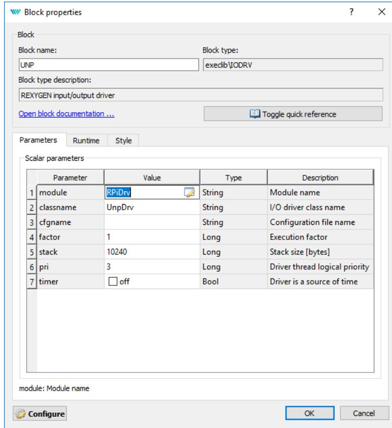
As the final step, rename the IODRV block to UNP, which will serve as a prefix for all I/O signals of this driver.
