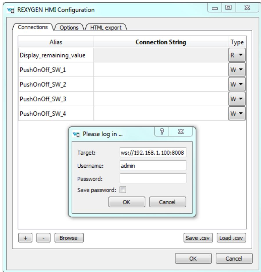
Select *Connection String* field of the `Display_remaining_value` item and afterwards browse the tree to the `TIMER_` block and **double-click** the `rt` parameter. The connection string of the parameter is copied to the `Display_remaining_value` alias, which is shown in the next figure.
