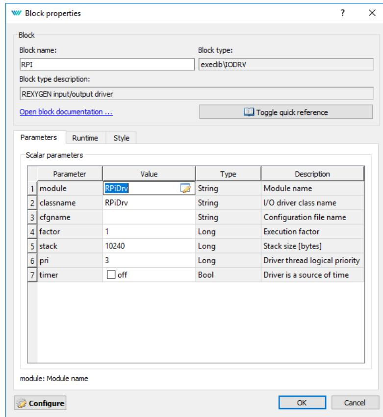
As the final step, rename the IODRV block to RPI, which will serve as a prefix for all I/O signals of this driver.
