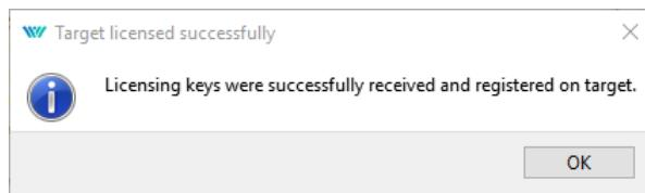
6. To check the licence, make sure the REXYGEN Studio is connected to the device and open the licensing dialog again (*Target → Licensing*). Check that the licence was applied correctly and that the RexCore runtime module no longer runs in demo mode.
