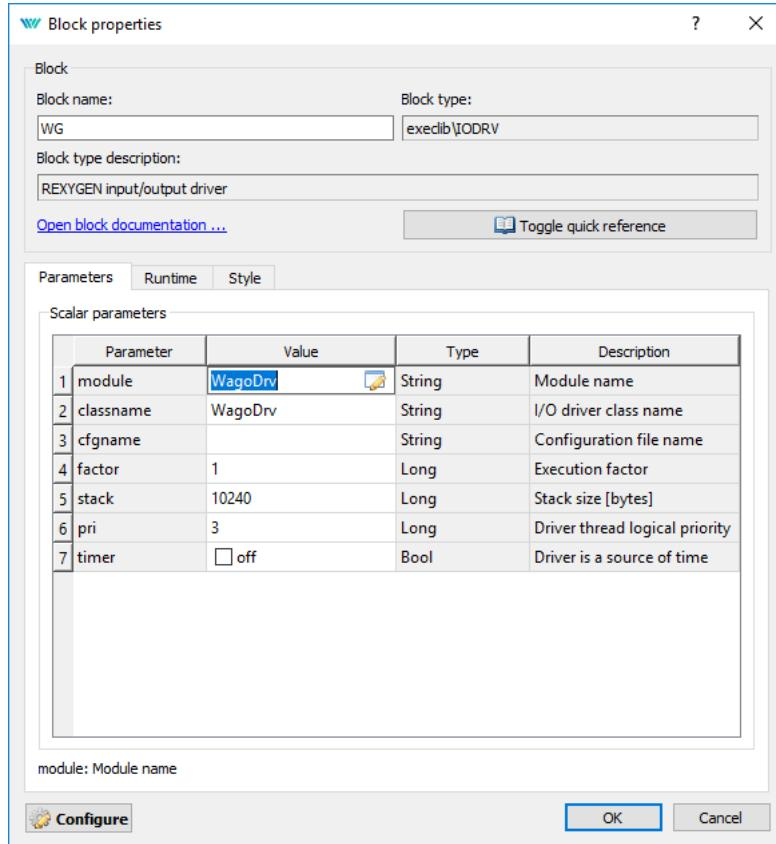
As the final step, rename the IODRV block to WG, which will serve as a prefix for all I/O signals of this driver.
