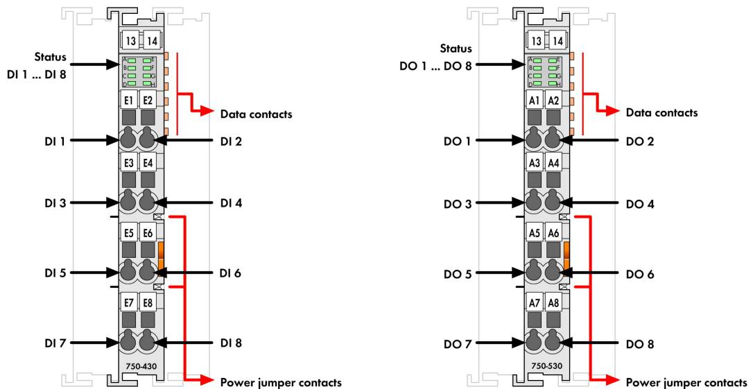
For details and wiring examples for WAGO PFC100/200 refer to documentation of the WAGO 750/753 modular I/O system.
