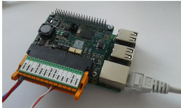
Figure 3.2: Terminal pinout for Monarco HAT.
