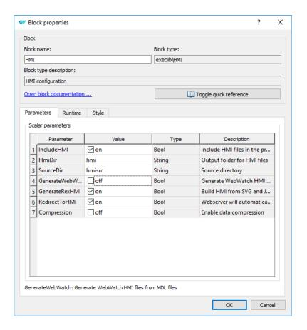
4. The HMI is now an integral part of your project. Compile the project again and you will see that the compile log contains more information. The index.html file is generated from the source index.hmi.js file. All the HMI files are generated into the hmi subfolder (HTML, JS and CSS files) and included in the resulting binary myproject\_exec.rex file.
