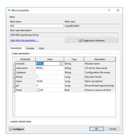
As the final step, rename the  ${\tt IODRV}$  block to RPI, which will serve as a prefix for all I/O signals of this driver.
