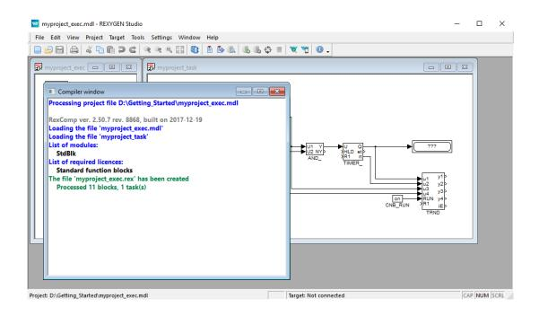
At this moment it is possible to deploy the control algorithm to the target platform. Use *Project/Compile and Download* in the menu or click the Compile and Download icon for this purpose. A dialog for defining the target device appears upon successful compilation.
