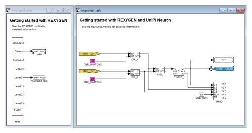
After compiling the project and downloading it to the UniPi Neuron the control algorithm interacts with the physical world. Again it is possible to switch to Watch mode and observe the signals in real-time or analyze the trends of signals. Flip the physical switches and watch the signals.
