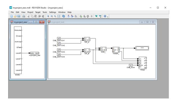
At this moment the executive configuration myproject\_exec.mdl and the corresponding myproject\_task.mdl file with the algorithm are ready. The algorithm will be evaluated in the direction of the arrows, starting from the source CNB blocks, passing through the OR\_, AND\_ and TIMER\_ blocks and finishing at the Display and TRND blocks.
