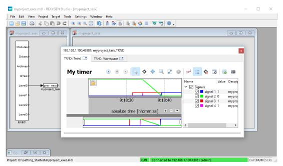
Try turning the CNB blocks off and change the pt parameter of the TIMER\_ block. Afterwards turn the CNB blocks on again and observe the signals in the TRND block again. As you can see, you can modify any parameter in real-time, which allows you to fine tune your algorithm.
