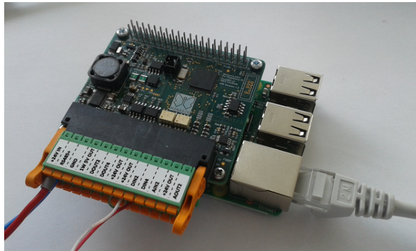
Figure 3.2: Terminal pinout for Monarco HAT.
